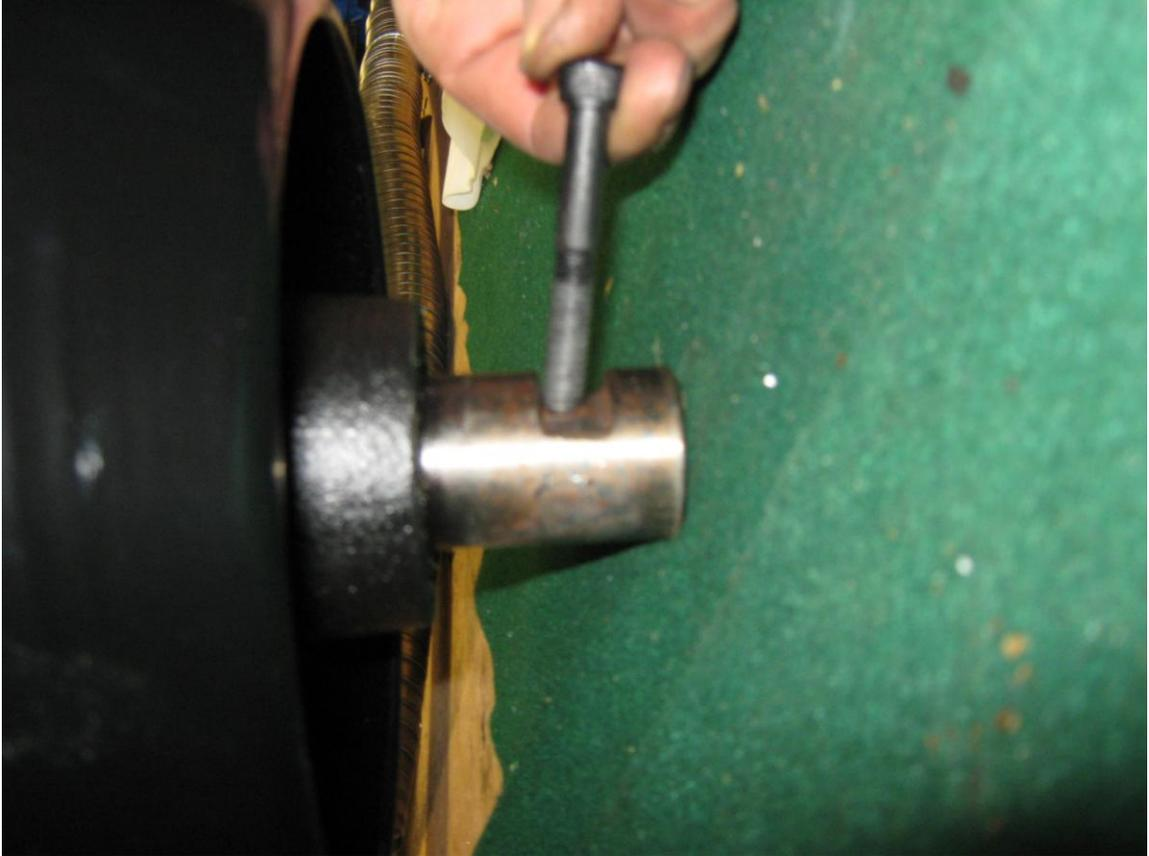
Look into the spindle socket- see where spindle bolt enters the socket. The spindle on the bottom of the head must be placed in such a way in socket that the cut-out on spindle lines up with the spindle bolt -since once that bolt is secure into the cut-out the head cannot come off. See photo 4 below.
